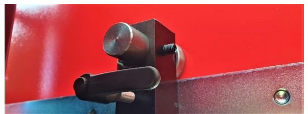
Detail of the stop with lever to block the cylinder in every position of the sliding lane
